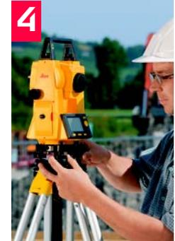
Use the foot screws of the tribrach to centre the plummet on the ground point. Ignore that the instrument is not yet levelled precisely.
