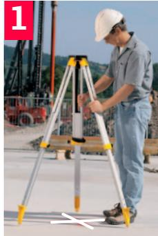
Extend the legs of the tripod so that they allow working in a comfortable posture. Position the tripod over the marked ground point, centering it as good as possible.
