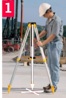
Extend the legs of the tripod so that they allow working in a comfortable posture. Position the tripod over the marked ground point, centring it as well as possible
