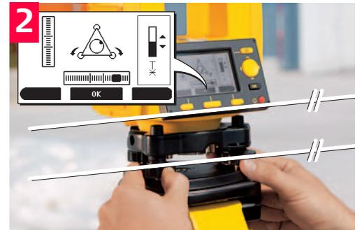
Center the electronic level of this axis by turning the two footscrews. Arrows show the direction for rotating the footscrews.
