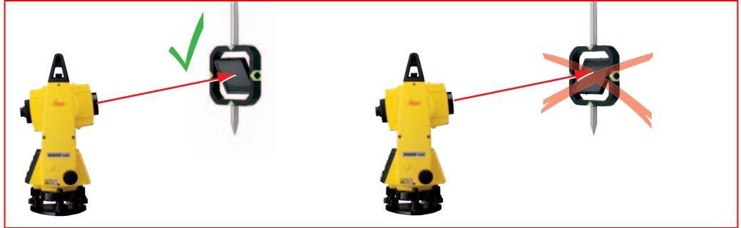
Tilt the moving part of the flat prism correctly.
