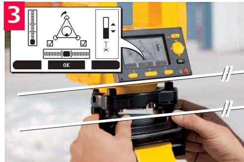
When the electronic level is centered the arrows are replaced by checkmarks.
