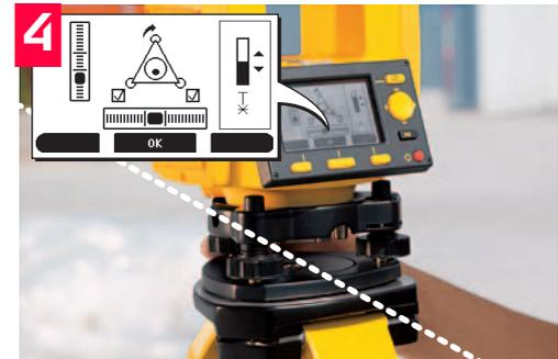
Center the electronic level for the second axis by turning the last footscrew. Arrows show the direction for rotating the footscrew.
