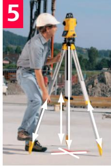
Adjust the legs of the tripod to level the circular level
