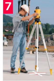
Centre the instrument precisely over the ground point by shifting the tribrach on the tripod plate.
